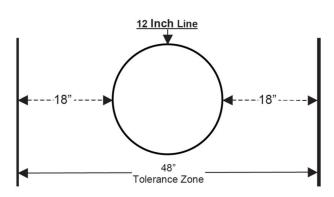
Tolerance Zone means the horizontal space within eighteen-inches of the outside wall or edge of the line or facility.
