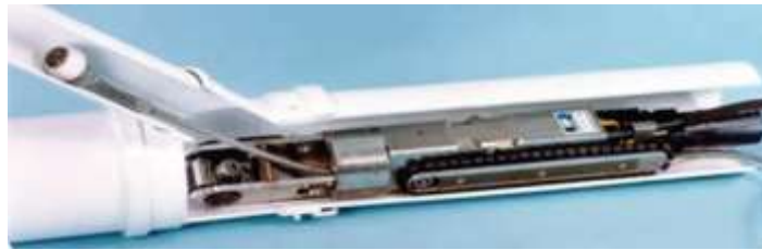
Figure 3 Lateral and Mainline Probe for Lateral Launch. Source Video Industrial Services
