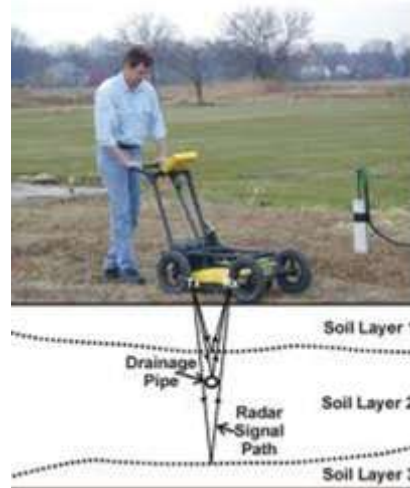
Figure 1 Example of Ground Penetrating Radar Equipment and Illustration of Results. Source USDA
