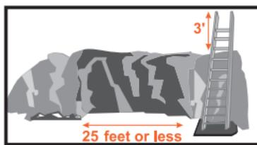
A competent person must inspect trenches daily and when conditions change. An unprotected trench is an early grave. Do not enter an unprotected trench.
