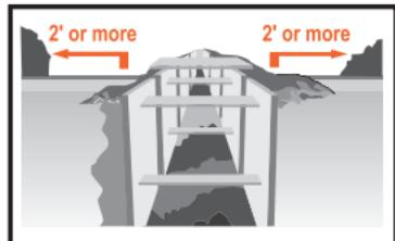
A safe way to exit must be provided within 25 feet of workers in a trench.
